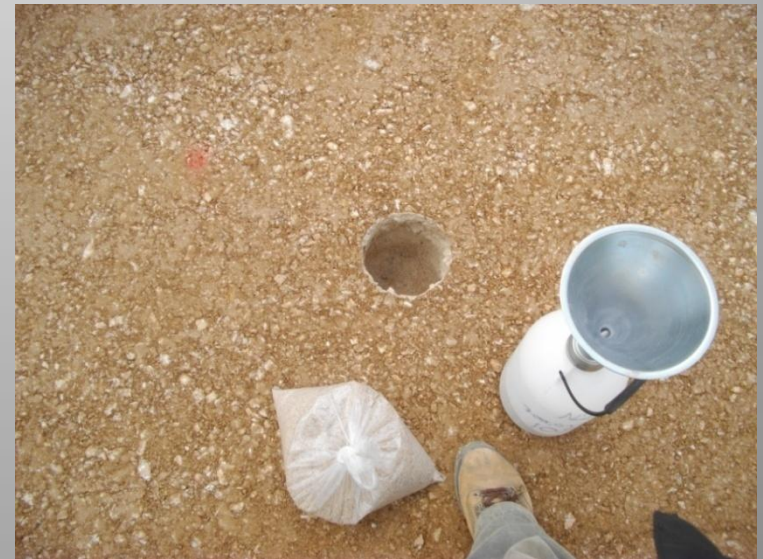
Compaction degree using Sand & Cone method
