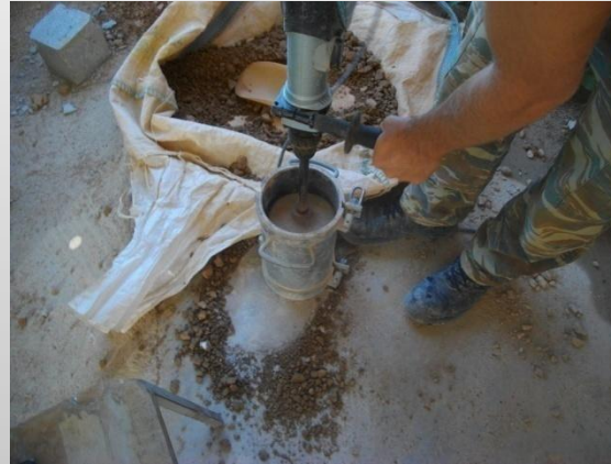
Compaction with a vibrating hammer
