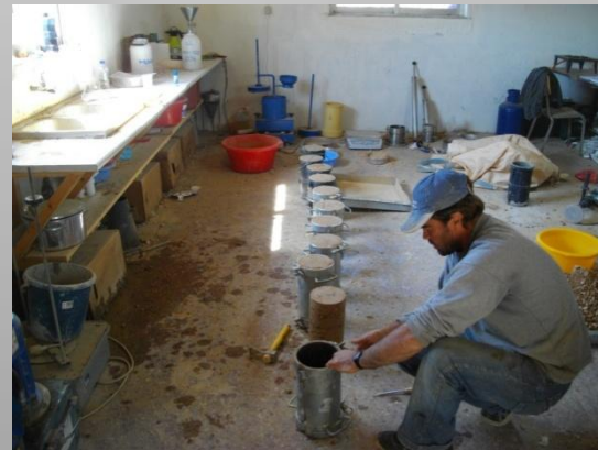
Molds with bond breaker for specimen removal
