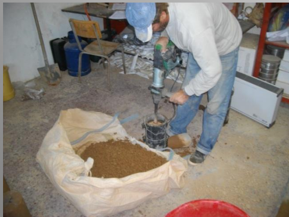
Molding lean rcc in cylindrical mold with a vibrating hammer
