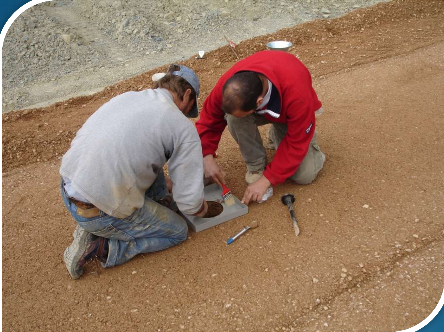
Compaction test on the trial section
