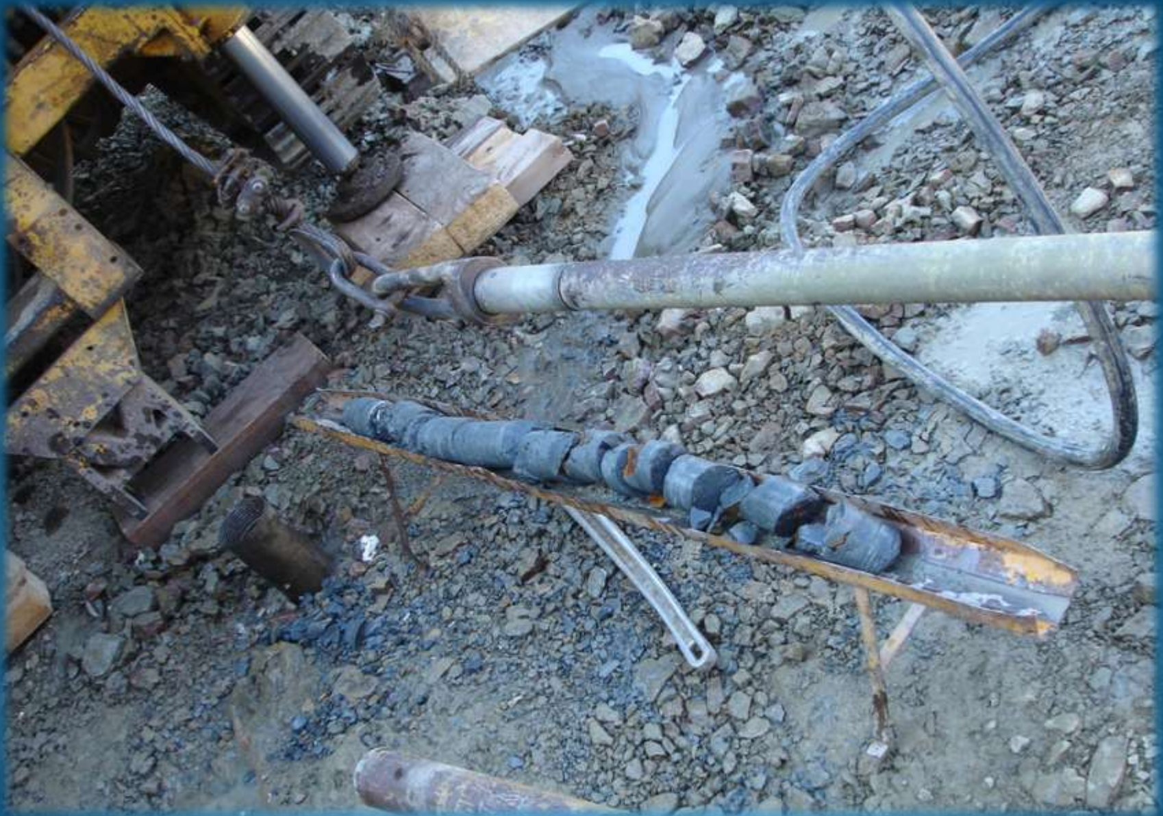
Ground core sampling
